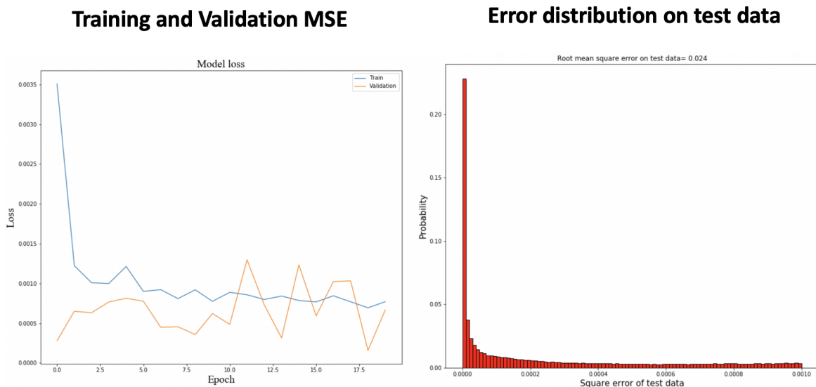
Figure 3: Left: Learning curve for MSE on train and validation data set. Both seems to converge after 15 epochs. Right: Squared error distribution on the test dataset. As seen in the figure, most of the error is very small. The y-axis is normalized to show probability.
